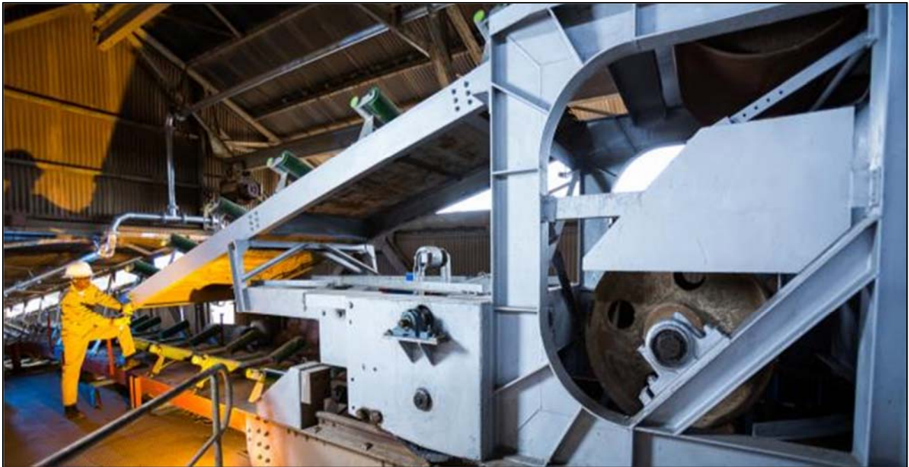
Figure 4: The new ore conveyor belt installed as part of Kipushi's upgrading work.
