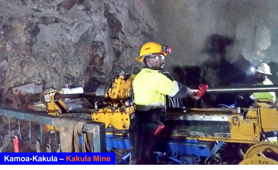
Drilling a cover hole at Kakula to analyze underground conditions for safe mine development.
