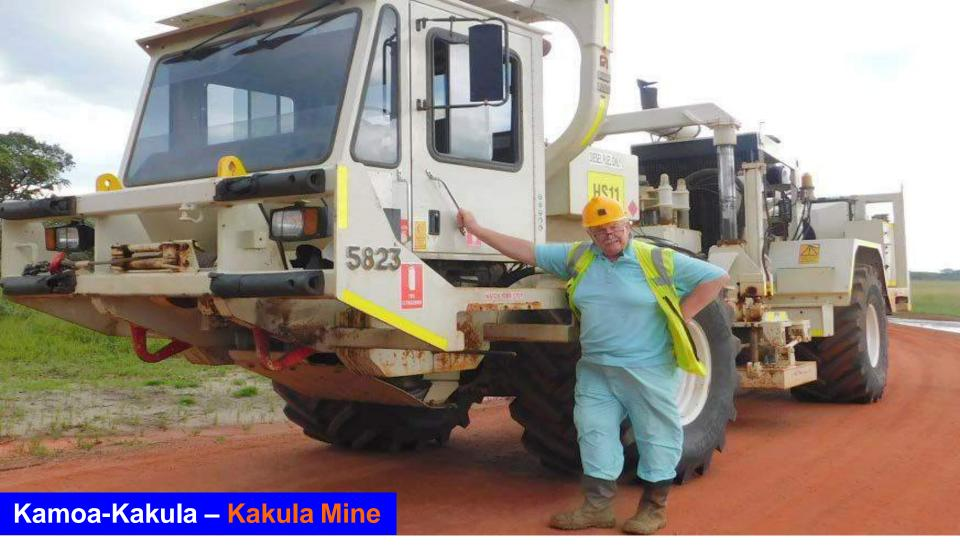
Victor Bridgett, Hi-Seis' Quality Control Manager, with a seismic vibrator rig being used to survey the Kamoa-Kakula licence area. The device creates seismic waves to produce reliable and quality images of hard-rock environments to help identify drilling targets to test for potential, new Kakula-like discoveries. Seismic work is being conducted by Hi-Seis, a leading international services company.
