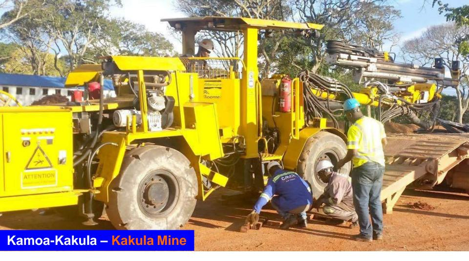
Delivery of a new jumbo drill rig to be used to expedite underground development work at the Kakula Deposit. Initial mine development is planned to begin at the deposit in a flat, near-surface zone along the deposit's axis that is between 7.1 and 11.7 metres thick, at a 3% cut-off, with copper grades of between 8.11% and 10.35%.
