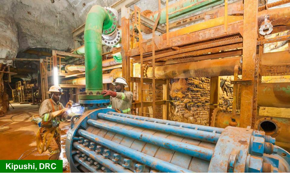
Regular maintenance of one of the Grifo pumps at the pump station at the mine's 1,200-metre level.
