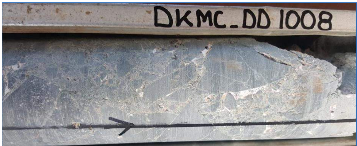
Figure 7.26 Typical Kakula Crackle Breccia From DKMC_DD1008
