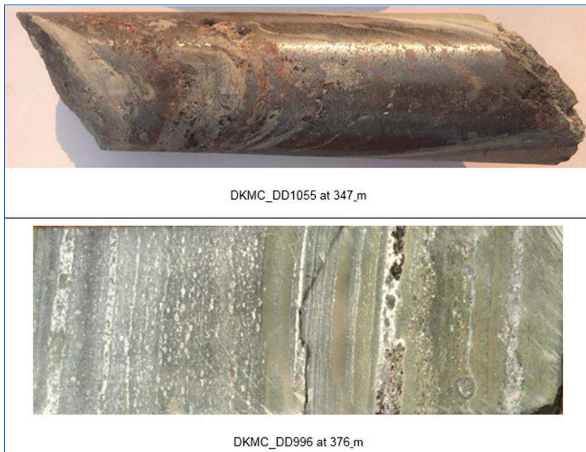
Figure 7.32 Examples of Coarse to Massive Chalcocite at Kakula
