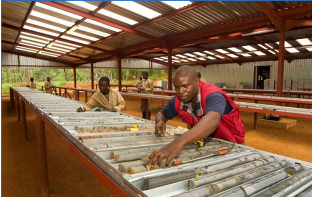
Figure 12.2 On-Site Core-Logging Facility
