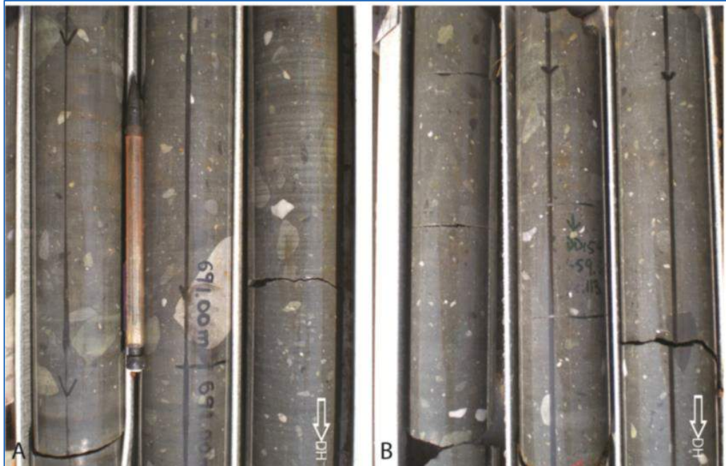
Figure 7.7 Clast-rich Diamictite (A) and Clast-poor Diamictite (B) DKMC_DD159
