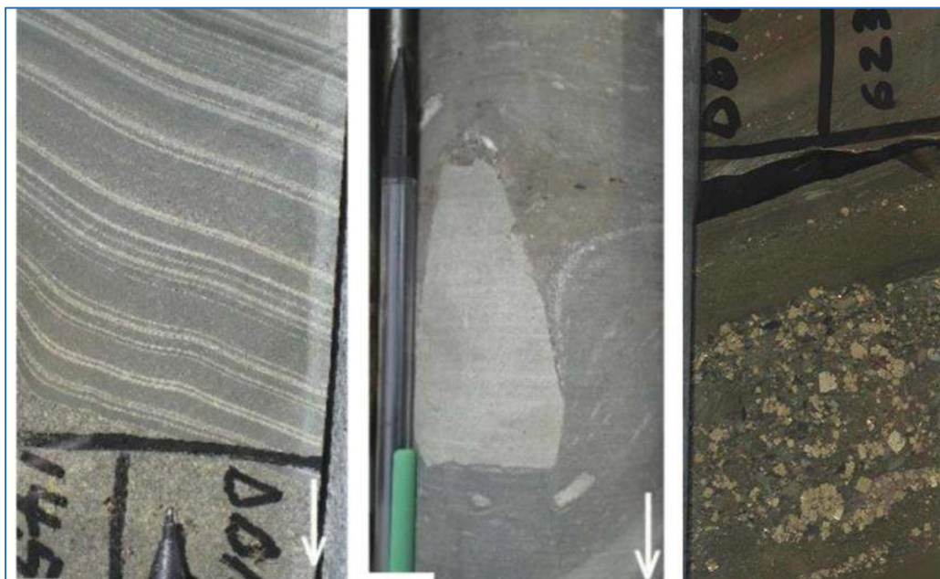
Figure 7.8 Distinctive Varves, Dropstone, and Pyrite at the Base of the KPS (DKMC_DD154)
