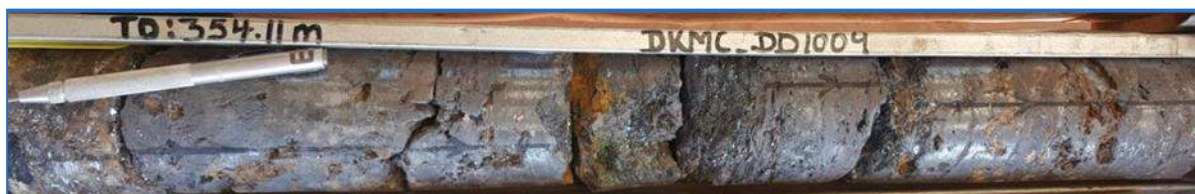
Figure 7.27 Massive Chalcocite Band Towards the Base of the Mineralised Zone in DKMC_DD1009 (at 354.1 m)
