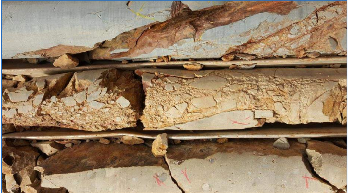
Figure 7.25 Steeply-Dipping Chaotic Breccia in DKMC_DD1015 (at 244.4 m)
