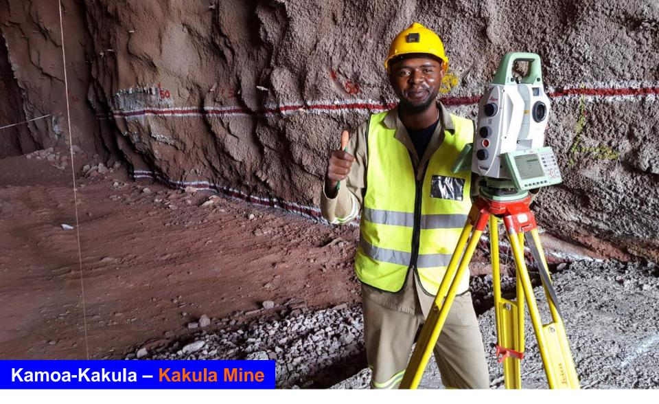
A mine geologist surveying the Kakula conveyor decline to ensure consistent grade and direction.
