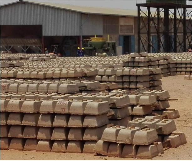
Heavy-gauge rails and concrete crossties (sleepers) being installed on a section of SNCC's main line from Lubumbashi to Sakania, at the Zambian border. The upgrading, financed by the World Bank, utilized crossties produced at a Lubumbashi plant. Similar components will be used on the planned upgrading of the spur line to the Kipushi Mine.
