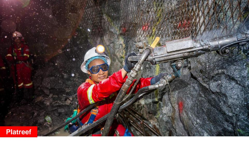
Platreef team member drilling as part of shaft-sinking support work in Shaft 1.
