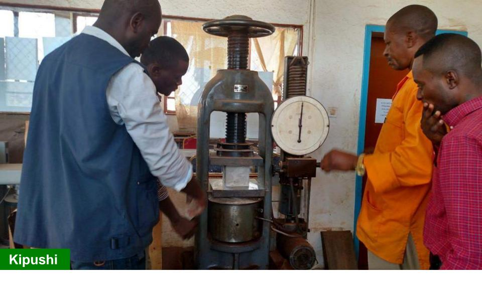
Testing the strength of a sample of concrete that will be used to construct the main underground haulage road on Kipushi's 1,150-metre level.
