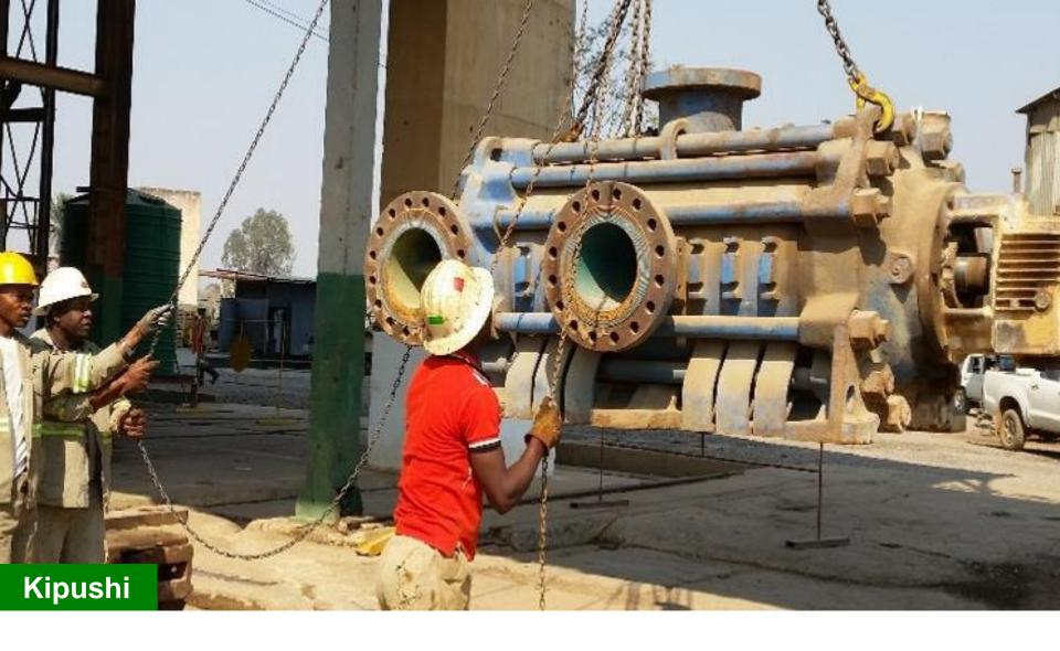
A high-capacity water pump brought to surface for upgrading.
