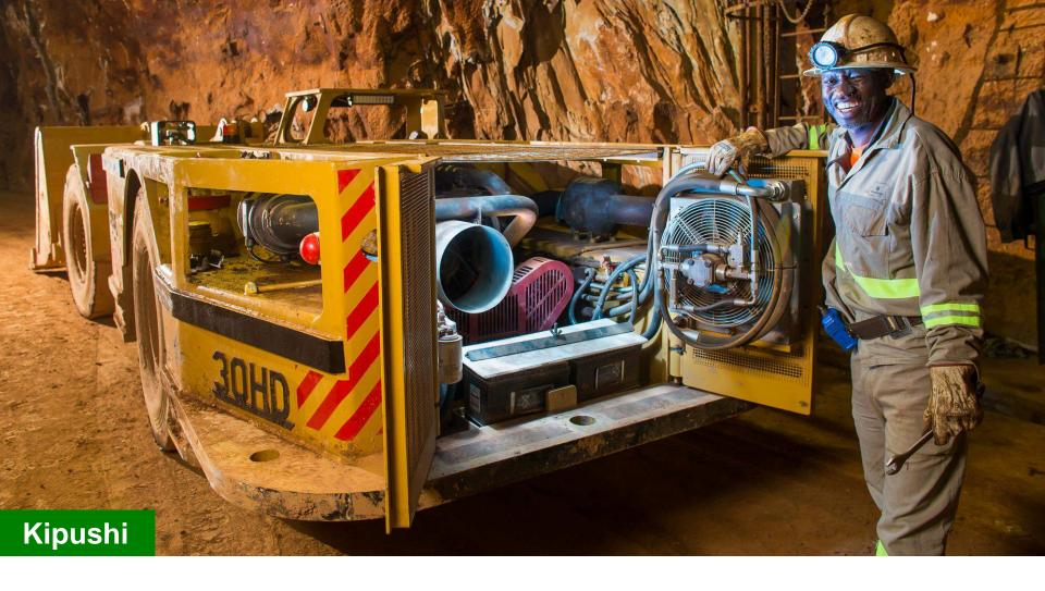
Inspection of a new underground scoop tram loader at Kipushi.
