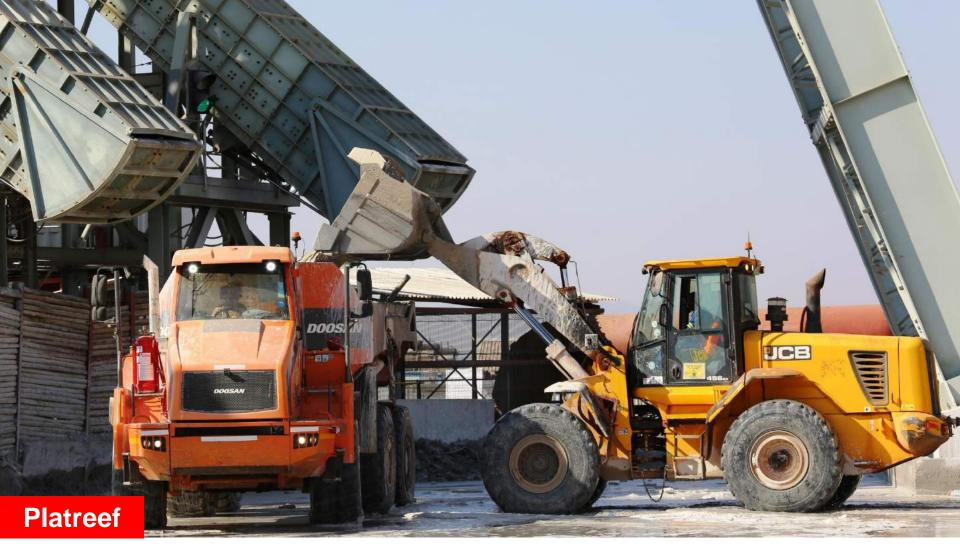
Removing rock excavated during current development of the 450-metre shaft station at Shaft 1. Shaft 1 will provide access to the Flatreef Deposit during the development of Shaft 2, the project's main production shaft.
