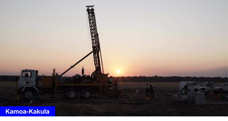
One of 14 rigs at Kamoa-Kakula, 10 of which are drilling in the Kakula/Kakula West area. Drill intercepts rich in chalcocite and bornite continue to be returned at Kakula West and Kakula. Drilling has extended the strike length of the Kakula West copperrich mineralized system to approximately 2.9 kilometres, and the total high-grade mineralized system to more than 12 kilometres.
