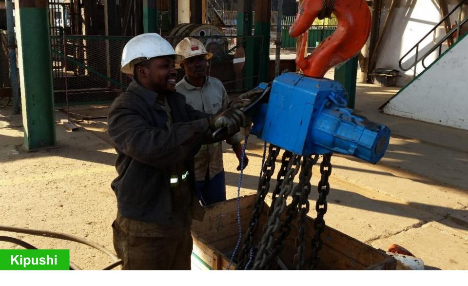
A 25-tonne hoist being overhauled as part of Kipushi's infrastructure upgrading program.
