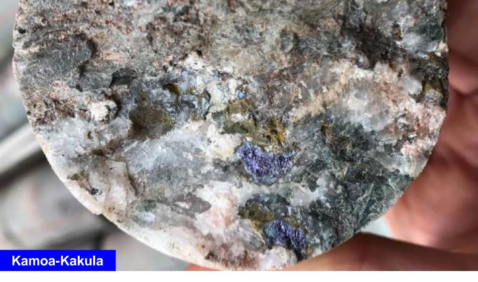
Bornite and chalcocite (both high-grade copper mineralization) in one of the drill holes at the Kakula West Discovery.
