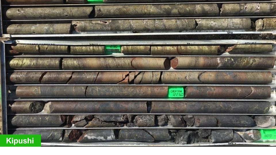
High-grade Kipushi drill core from the current underground drill program showing massive chalcopyrite (copper-rich) and massive honey sphalerite (zinc-rich, with silver and germanium) from the Southern Zinc Zone. The 6,500-metre drilling program included metallurgical holes into the Big Zinc Zone and resource expansion holes in the Fault Zone and the Nord Riche and Southern Zinc zones.
