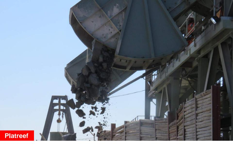
Broken rock from shaft-sinking operations being delivered to the surface from the bottom of Shaft 1.
