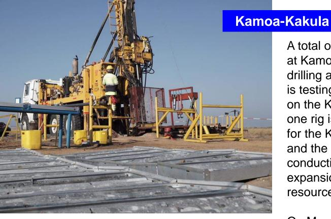
A total of 16 rigs are drilling at Kamoa-Kakula. Seven rigs are drilling at Kakula West; one rig is testing exploration target areas on the Kamoa-Kakula Project; one rig is drilling geotechnical holes for the Kakula box cut; and the remaining rigs are conducting resource upgrading and expansion drilling in the Kakula resource area.
