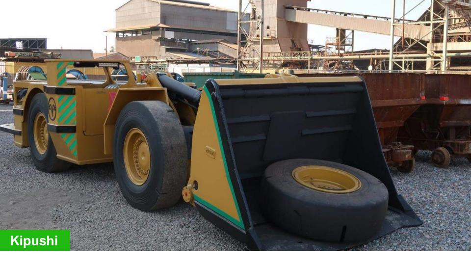
A new underground scooptram loader at Kipushi's Shaft 5 being prepared to be lowered underground.
