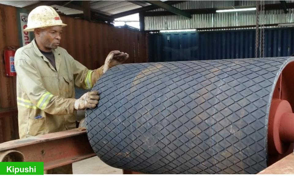
Upgraded pulley for Shaft 5 conveyor. Engineering work at the Kipushi Project has focused on the upgrading of Shaft 5 conveyances and infrastructure.
