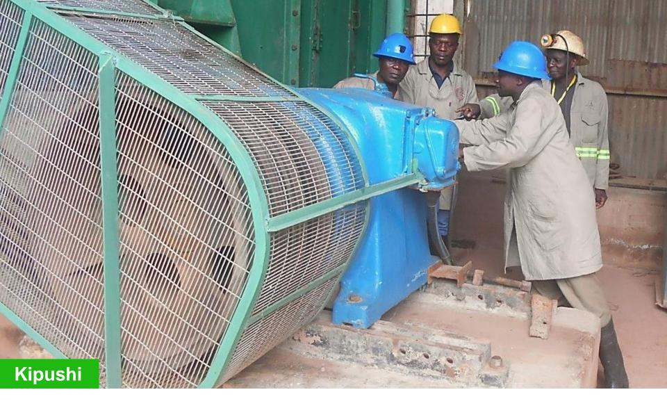
A new, high-volume ventilation fan has been installed on surface at Kipushi's Shaft 4 to provide fresh air underground.
