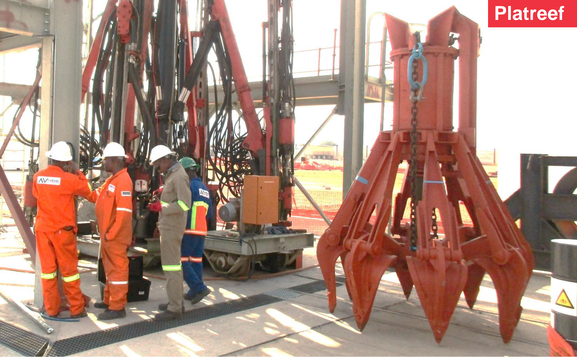
Jumbo drill rig and vertical shaft mucker used for the main shaft sinking at Shaft 1.
