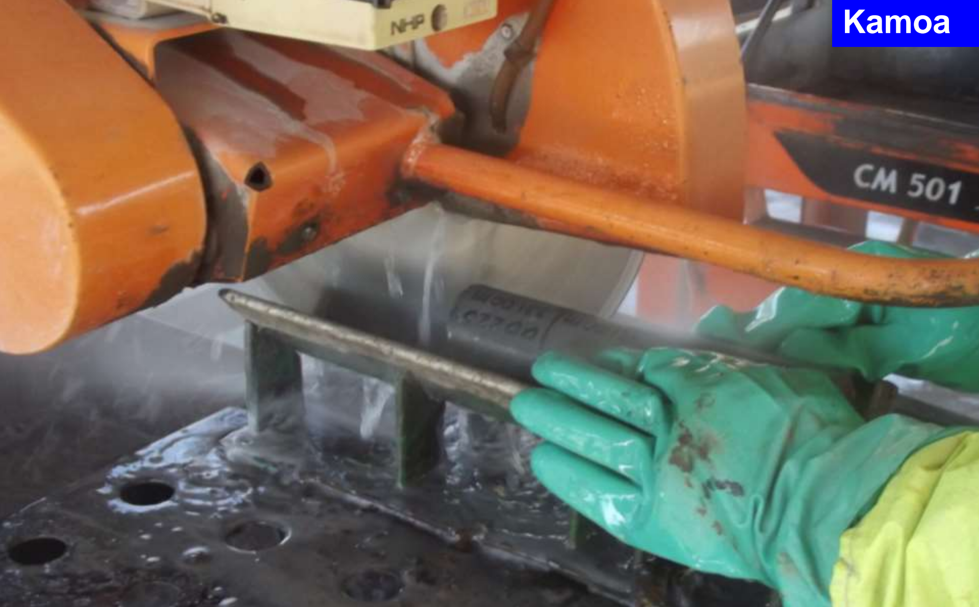
Cutting Kakula drill core in preparation for assaying.
