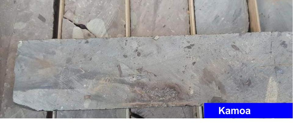
Core from Kakula drill hole DD1026 showing high-grade chalcocite mineralization. DD1026 intersected 14.66 metres (true width) of 7.66% copper at a 3.0% copper cut-off, beginning at a downhole depth of 333.8 metres; 15.48 metres (true width) of 7.39% copper at a 2.5% copper cut-off; 16.97 metres (true width) of 6.94% copper at a 2.0% copper cut-off; and 18.57 metres (true width) of 6.49% copper at a 1.0% copper cut-off.
