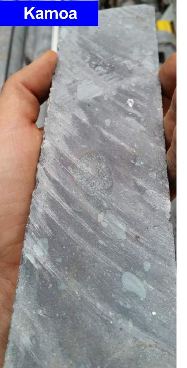
Core from Kakula drill hole DD1016 showing high-grade chalcocite mineralization (chalcocite is approx. 80% copper by weight). DD1016 intersected 8.75 metres (true width) of 9.84% copper at a 3.0% copper cut-off, beginning at a downhole depth of 362.0 metres; 9.27 metres (true width) of 9.11% copper at a 2.5% copper cut-off; 10.22 metres (true width) of 8.49% copper at a 2.0% copper cut-off; and 18.78 metres (true width) of 5.32% copper at a 1.0% copper cut-off.
