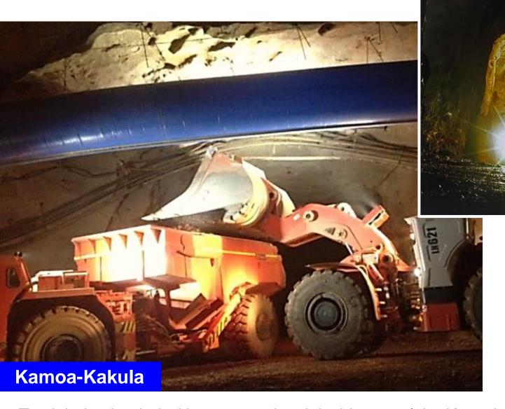
Truck being loaded with excavated rock inside one of the Kansoko Mine's two decline tunnels.
