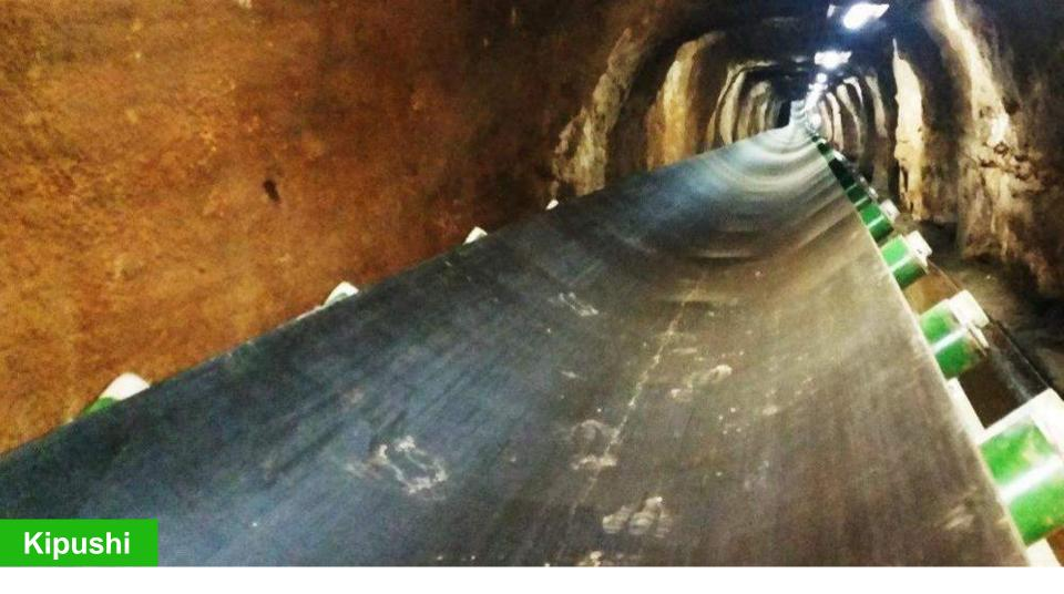
The new ore conveyor belt installed at 1,150-metre-level as part of Kipushi's infrastructure upgrading program.
