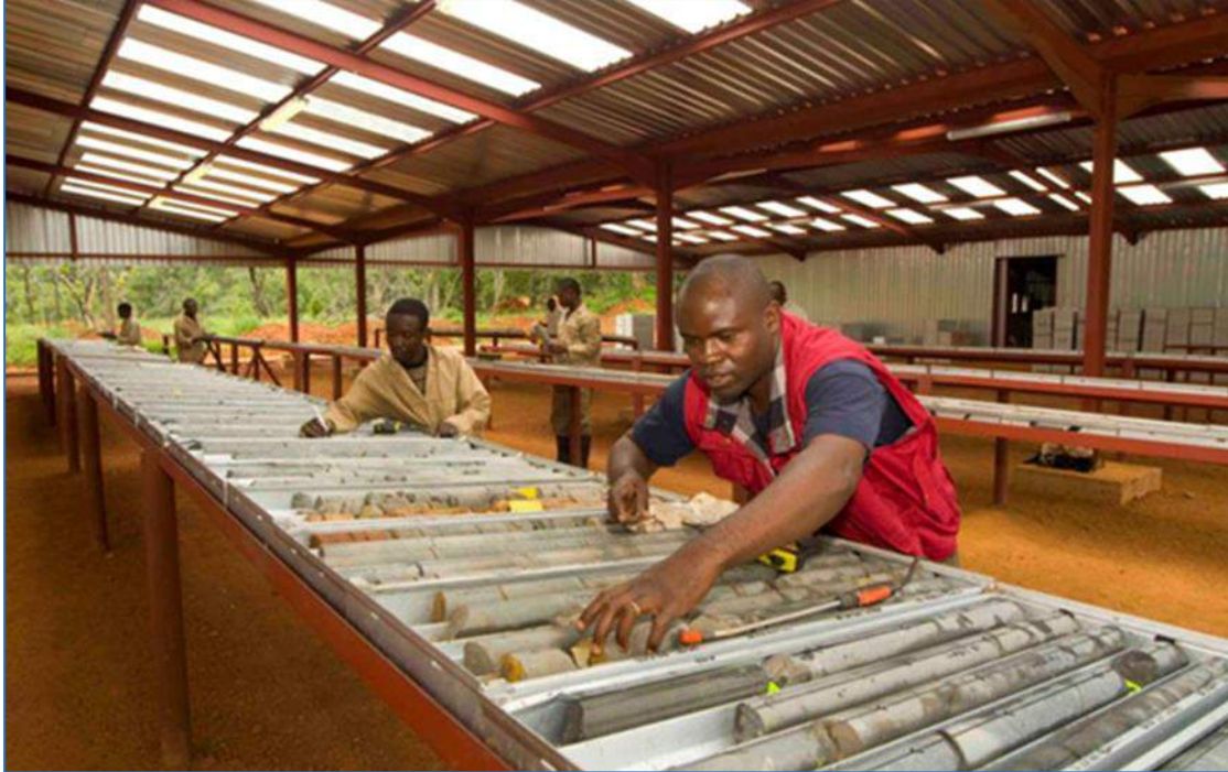
Figure 12.2 On-Site Core-Logging Facility
