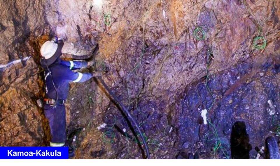
A Byrnecut contractor loading explosives in preparation for a blast at one of the Kansoko Mine's twin declines.
