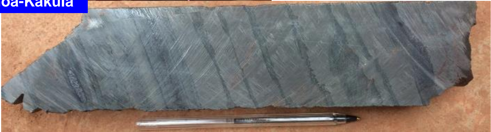
High-grade copper core sample from a newly completed Kakula drill hole showing disseminated-banded chalcocite.
