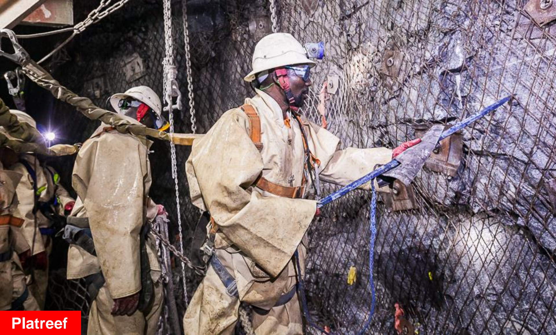
Platreef shaft-sinking crew checking the shaft sidewall for loose material.
