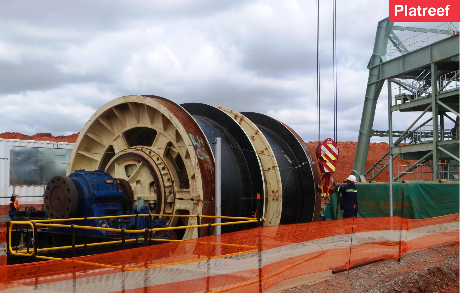
Shaft 1 kibble winder, which is being used to remove blasted rock from the bottom of Shaft 1 during the initial sinking operations
