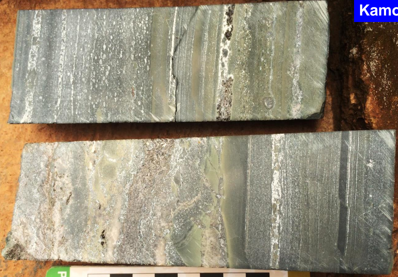
Finely disseminated chalcocite within bedded sandstone-siltstone. Sample grades at 15% copper from 375.45 metres to 376.00 metres in Kakula drill hole DD996
