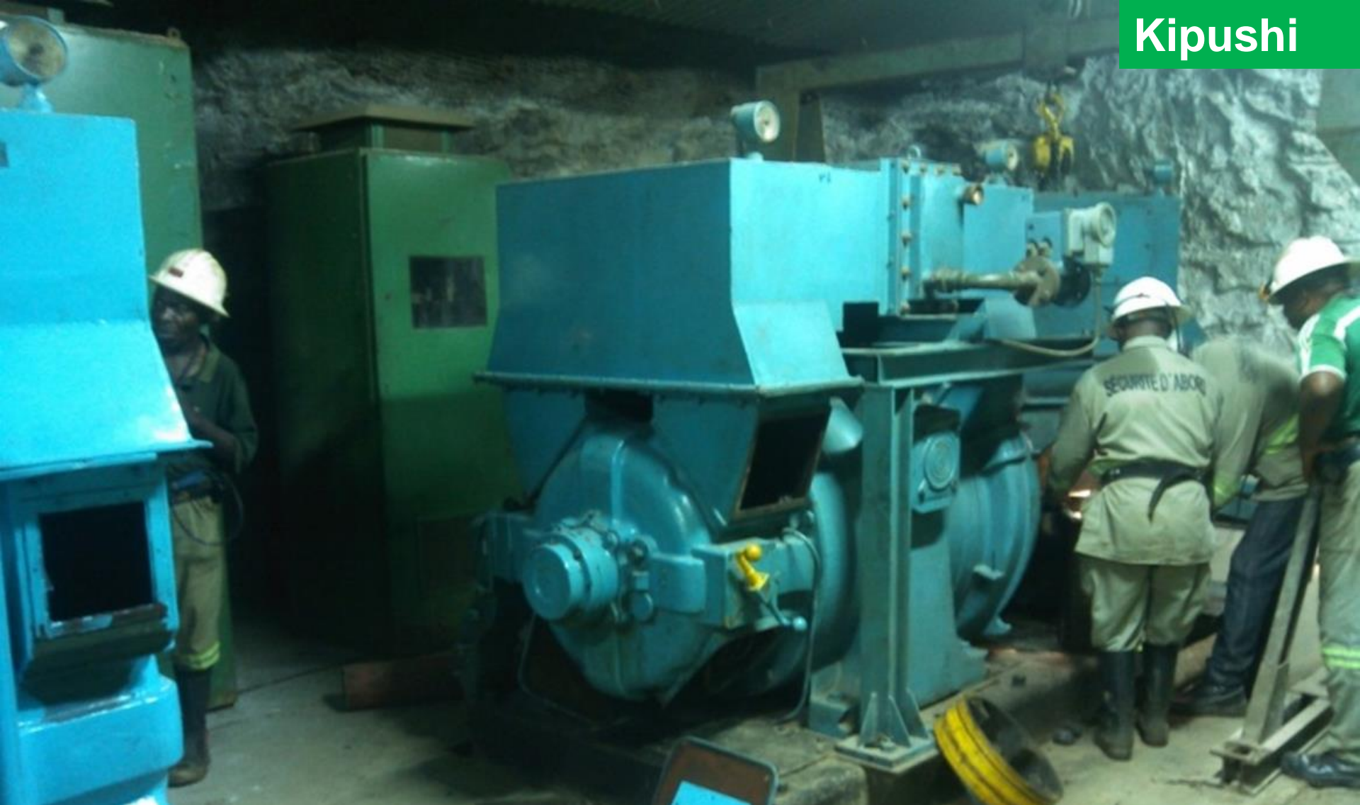
Generator rectifier for an underground winder, 450 metres below surface
