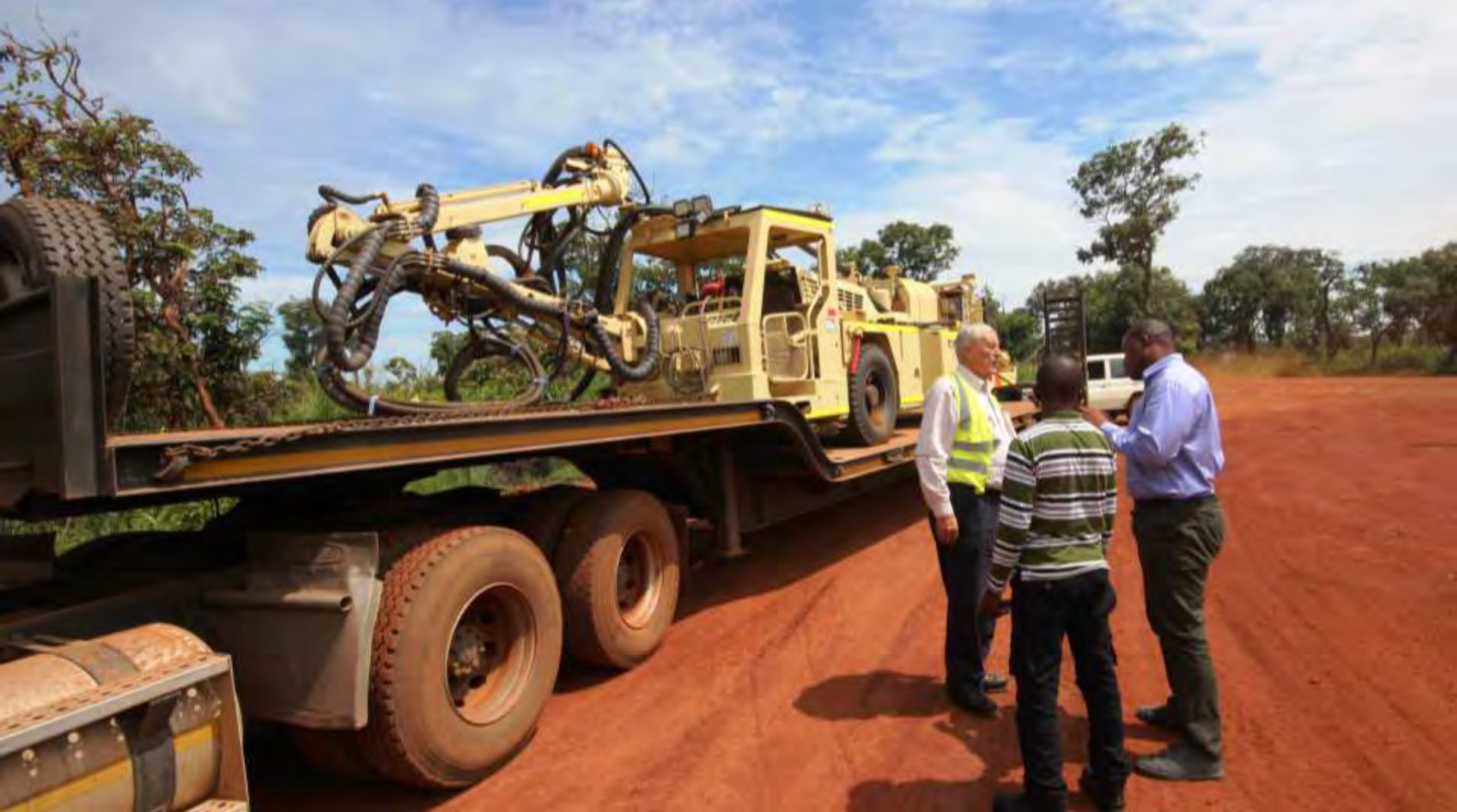
Arrival of the shotcrete machine for decline development
