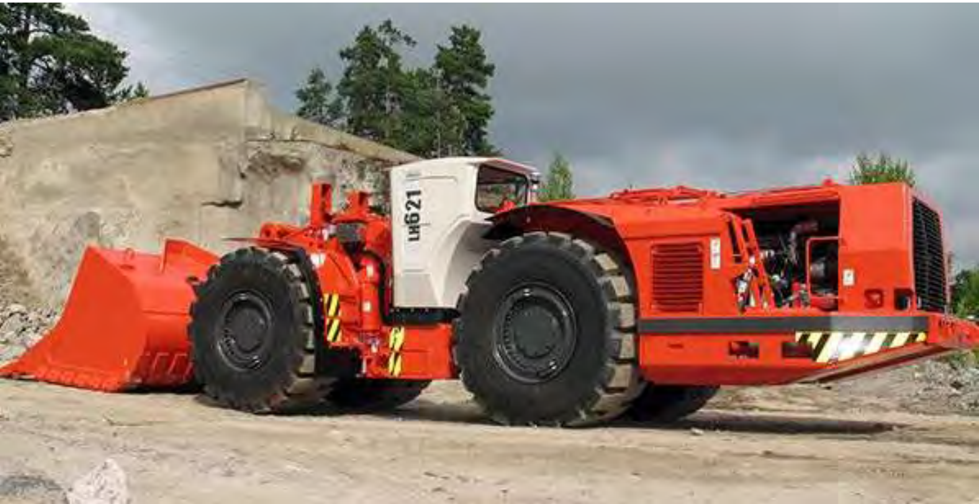
Sandvik LH-621 scooptram, the type of machine that will be used for decline development
