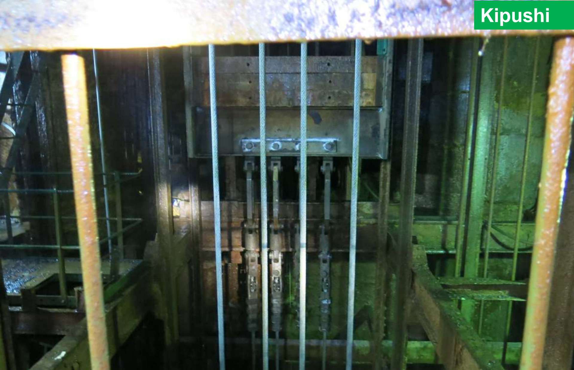
New wire ropes installed for counterweight at the 1,200-metre station in Shaft 5.
