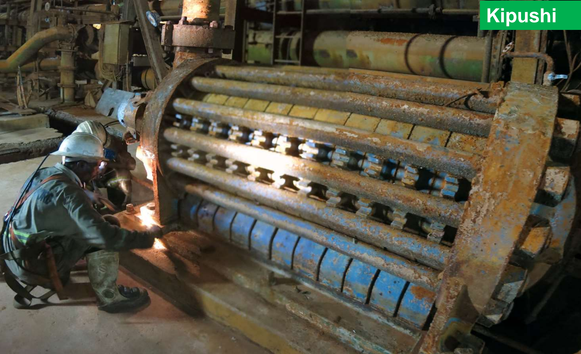
Cleaning the Grifo pump at the 1,200-metre pump station.
