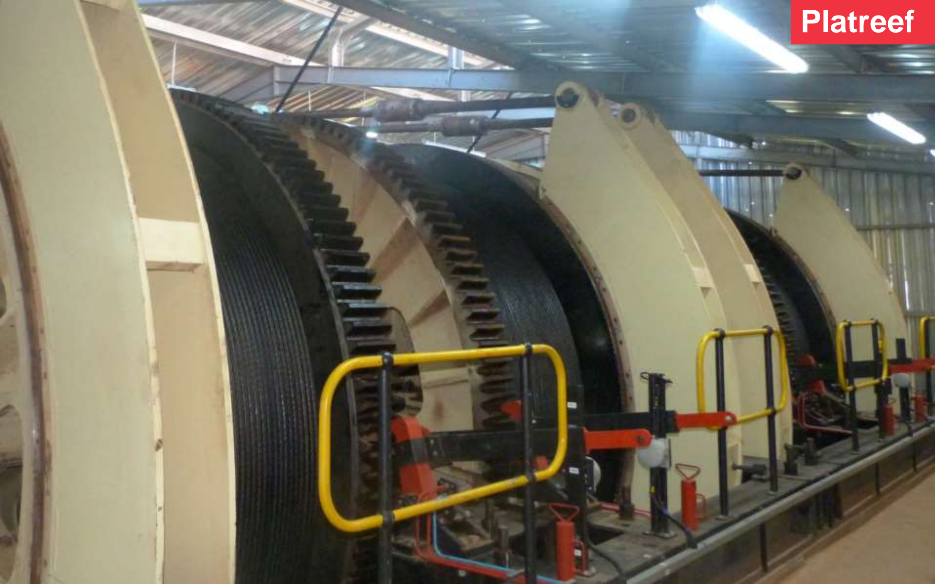
Shaft 1 stage winder completed for licencing inspection by the Department of Mineral Resources.
