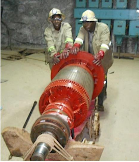
Workers upgrading a pump motor and preparing it for installation on the mine's 450-metre level.
