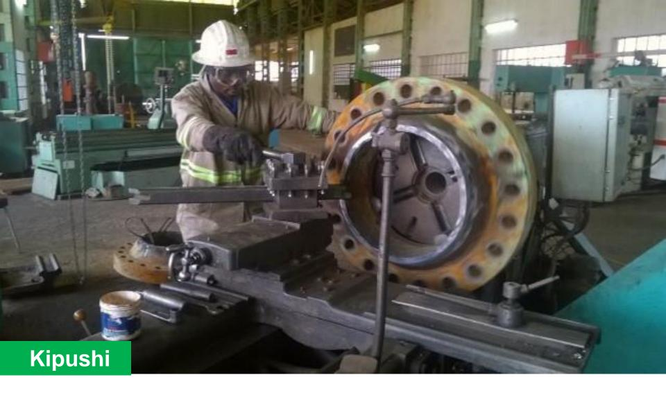
A mechanic machining a pump flange as part of the upgrading of existing underground mining equipment installed at Kipushi.
