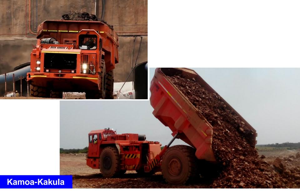
Excavated rock from the declines being hauled to the surface and tipped.
