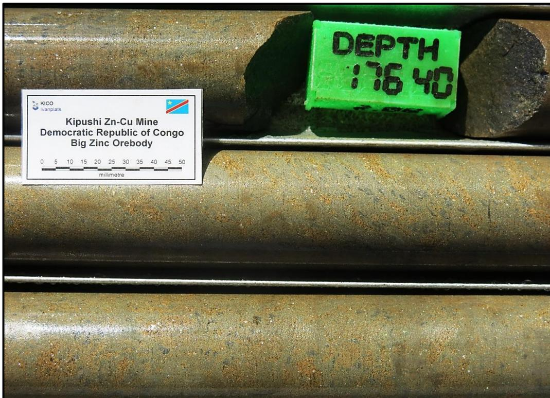
**Core from KPU004, the first hole drilled in the Série Récurrente zone on Kipushi's northern limb, which intersected a 15-metre, copper-rich mineralized zone.**
