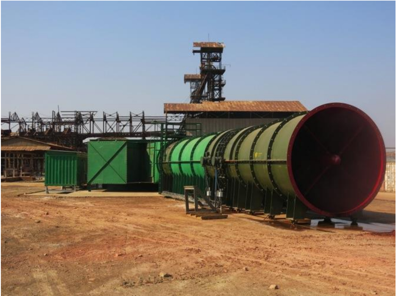
Figure 14: New, main ventilation fan at Shaft #4, fabricated on site and operational.
