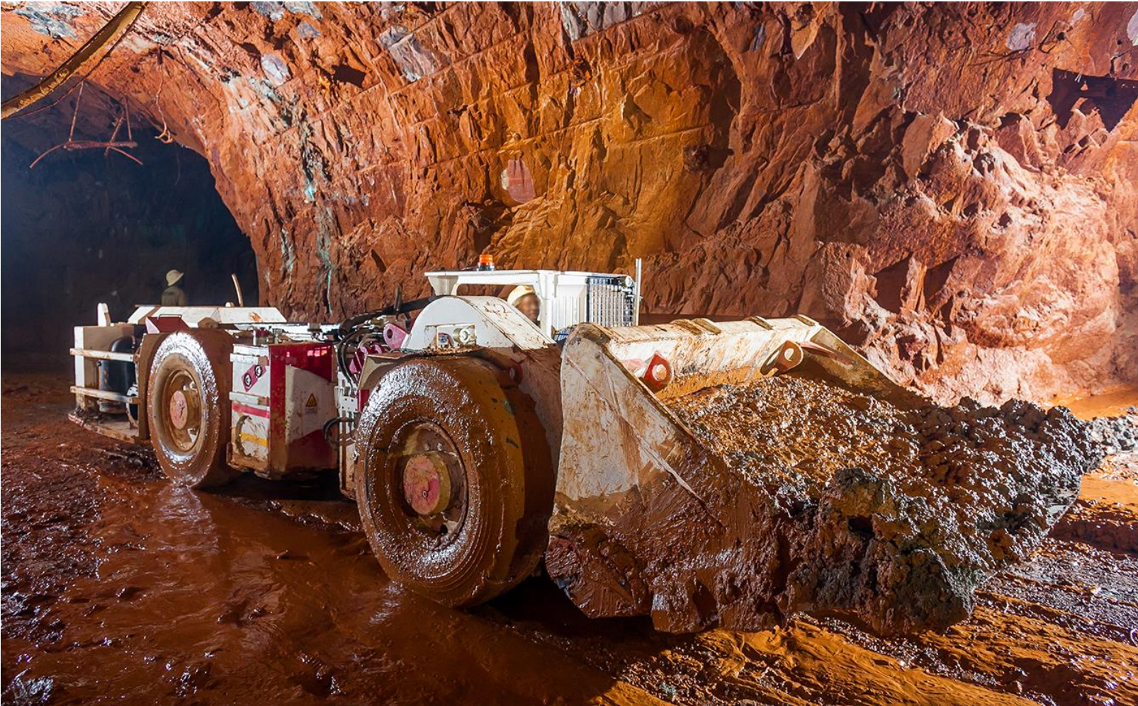
Figure 11: Scooptram removing mud from access on 1,150-metre level.
