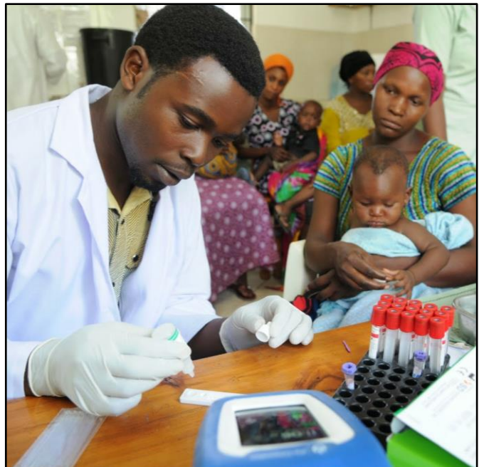
Photo 1: Fio’s Deki Reader introduces a new dimension in malaria detection, helping to deliver a rapid, accurate diagnosis and transmitting results to a cloud database.
