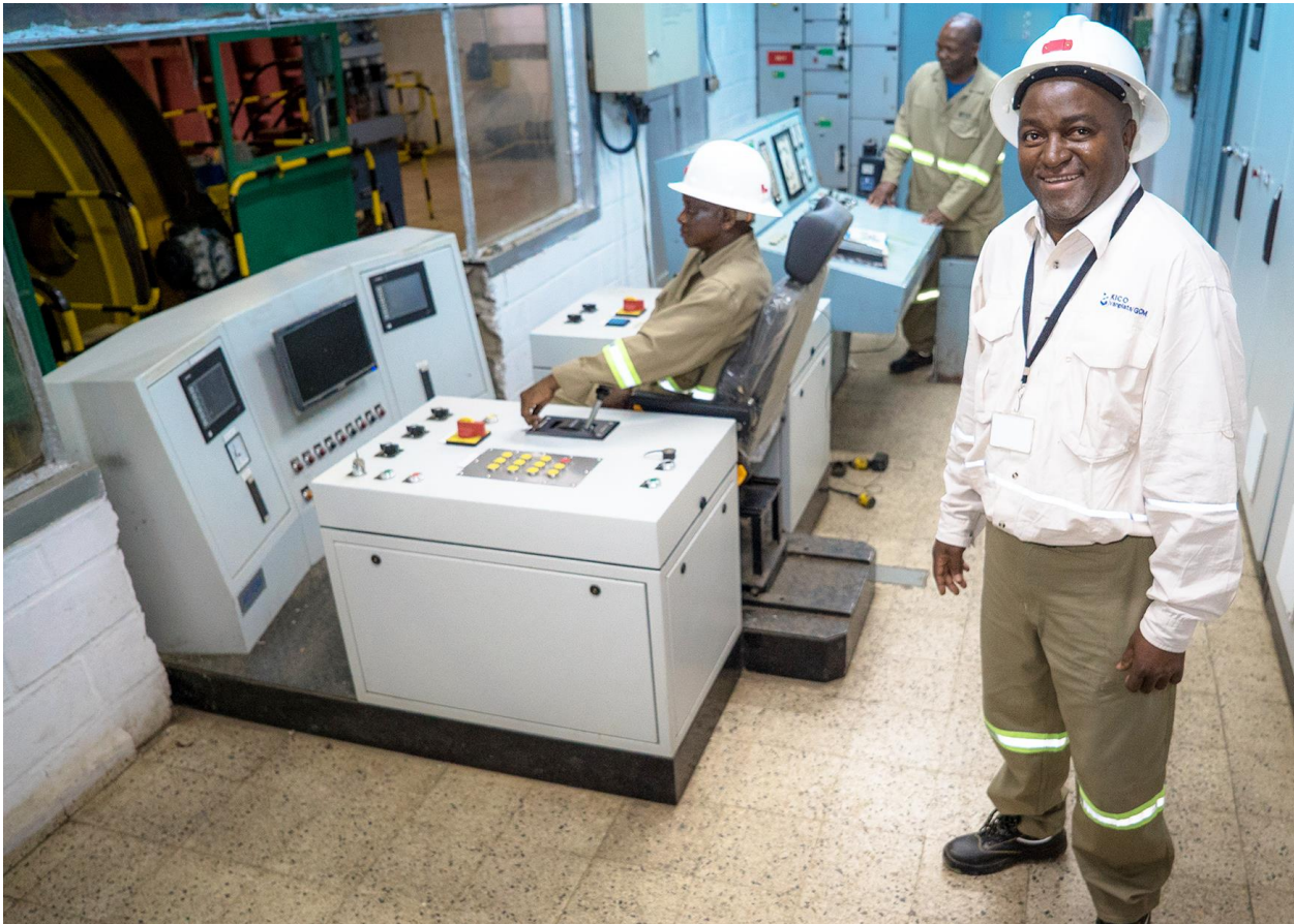
Figure 11: New winder control centre at Shaft 5.
