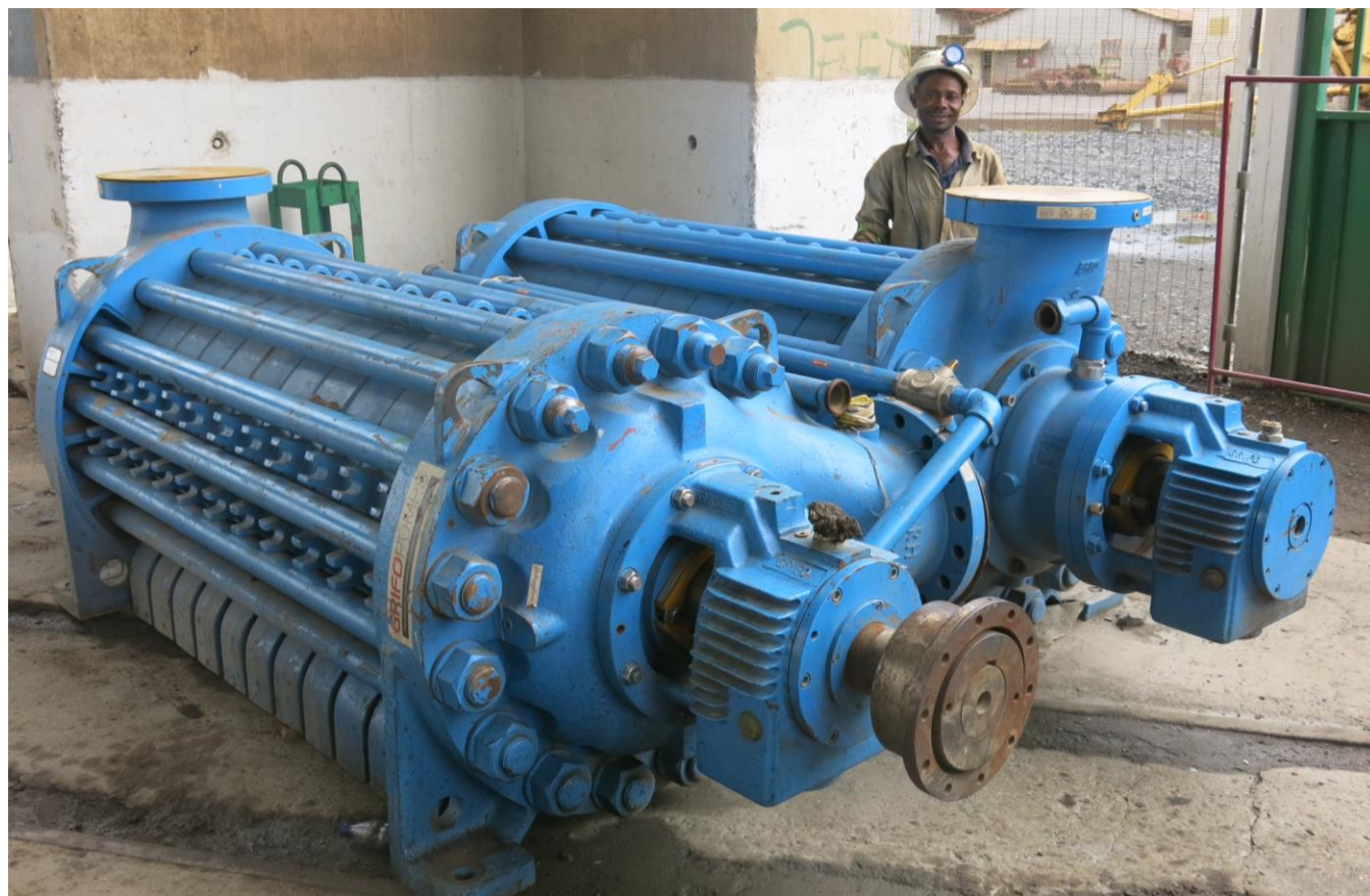
Figure 7: Two of three new high-volume Grifo pumps to be installed at the main pumping station 1,210 metres below surface.
