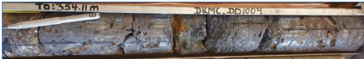
Figure 7.23 Massive Chalcocite Vein Towards the Base of the Mineralised Zone in DKMC_DD1009 (at 354.1 m)
