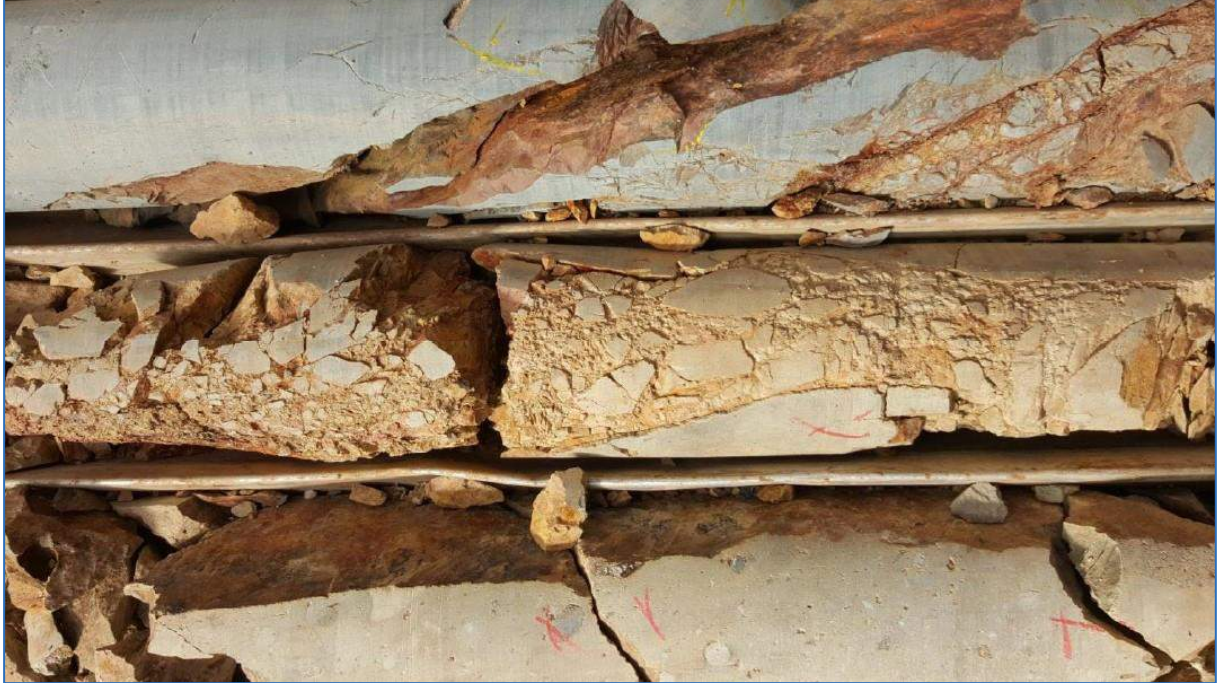
Figure 7.21 Steeply-Dipping Chaotic Breccia in DKMC_DD1015 (at 244.4 m)
