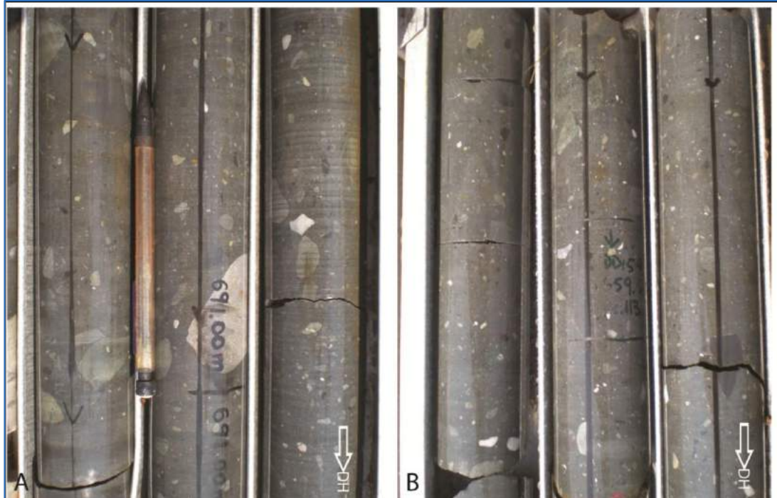
Figure 7.6 Clast-rich Diamictite (A) and Clast-poor Diamictite (B) DKMC_DD159
