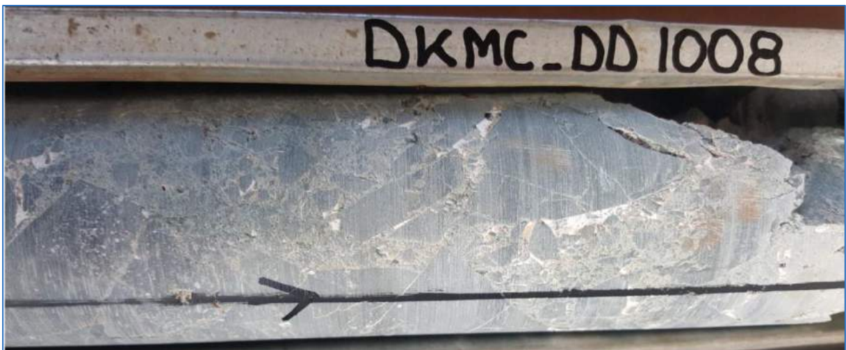
Figure 7.22 Typical Kakula Crackle Breccia From DKMC_DD1008
