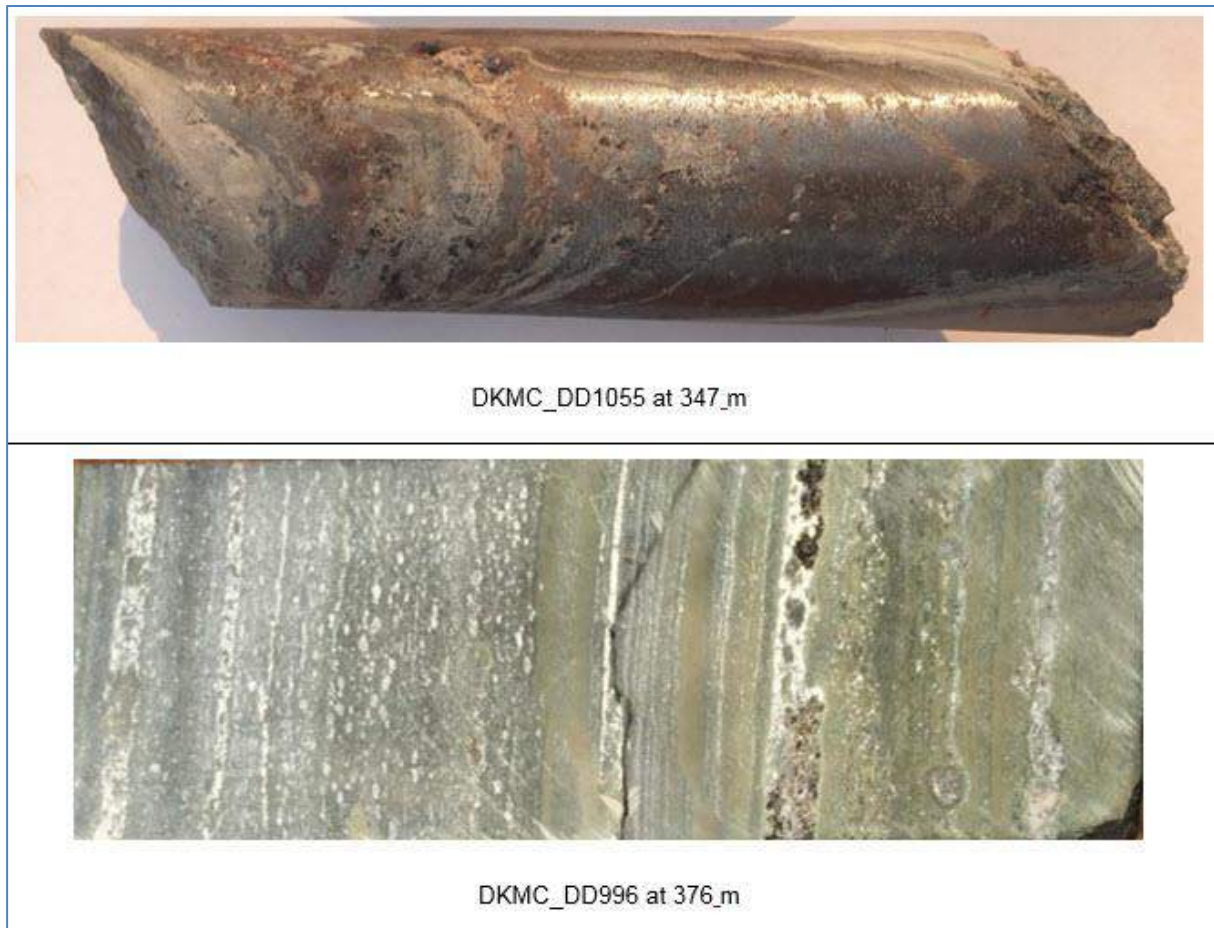
Figure 7.29 Examples of Coarse to Massive Chalcocite at Kakula
