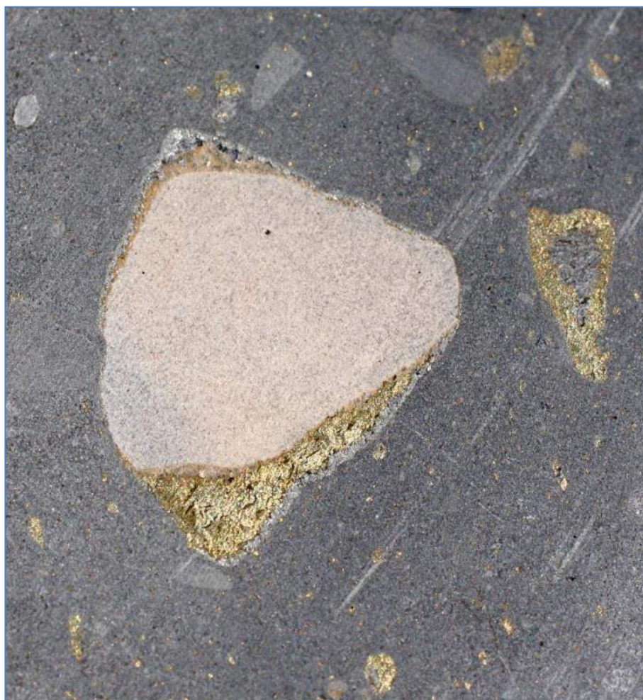
Figure 13.21 Typical Kamoā Hypogene Mineralisation in Diamictite
