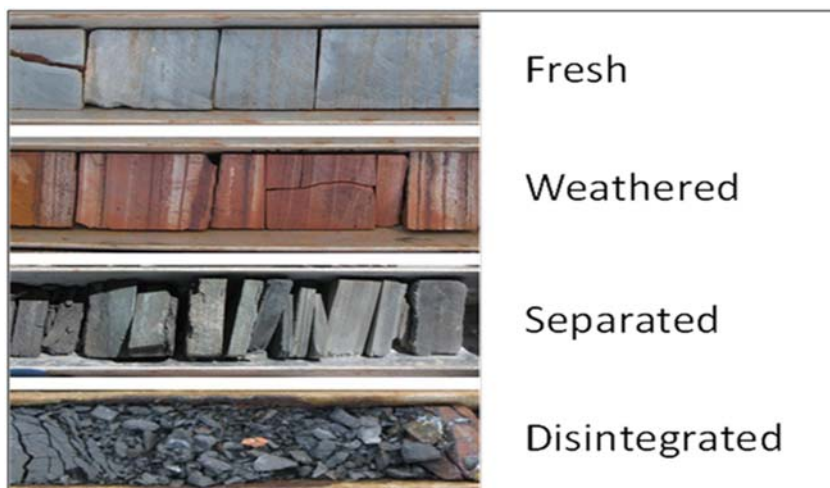
Figure 16.4 Representative Core Photos showing KPS Geotechnical Weathering Categories
