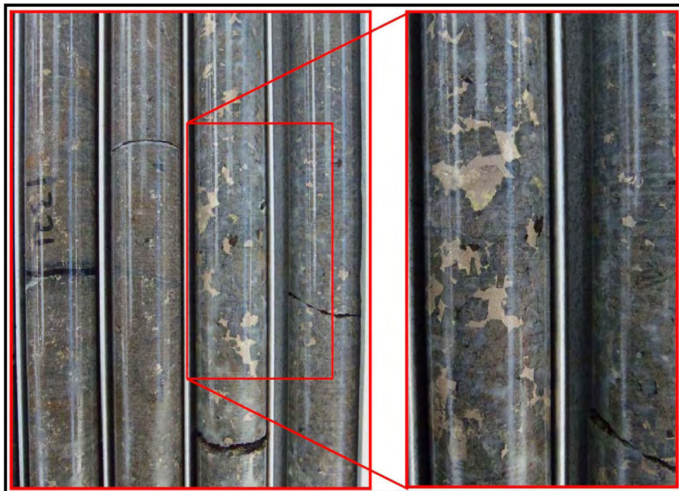
Figure 7-22: Core Photograph from UMT083 at 1,323 m Depth, Illustrating Sulphide Mineralization
