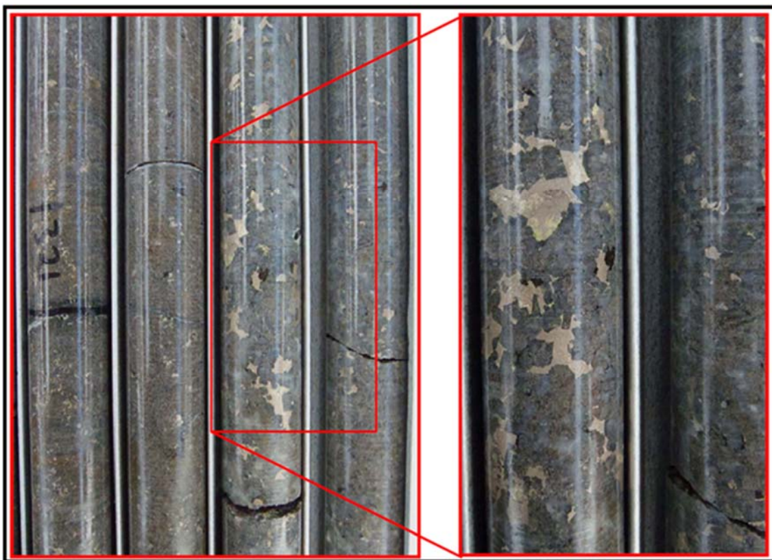
Figure 7.23 Core Photograph from UMT083 at 1,323 m Depth, Illustrating Sulphide Mineralization
