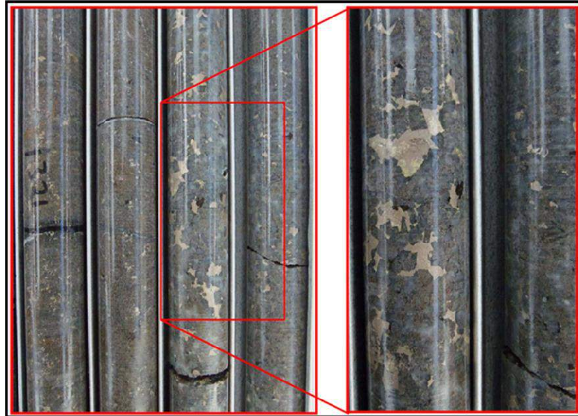
Figure 7.23 Core Photograph from UMT083 at 1,323 m Depth, Illustrating Sulphide Mineralisation
