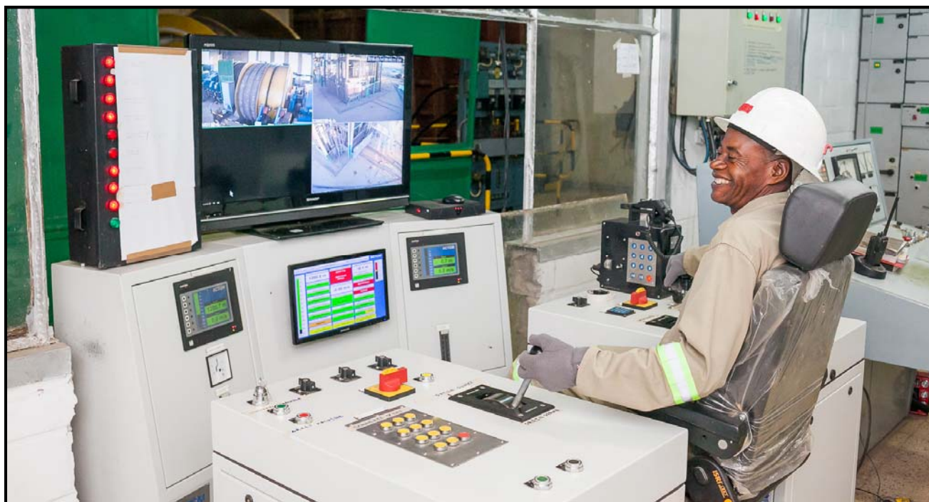
Figure 5: Shaft 5 hoist operator at new control panel with CCTV monitors.
