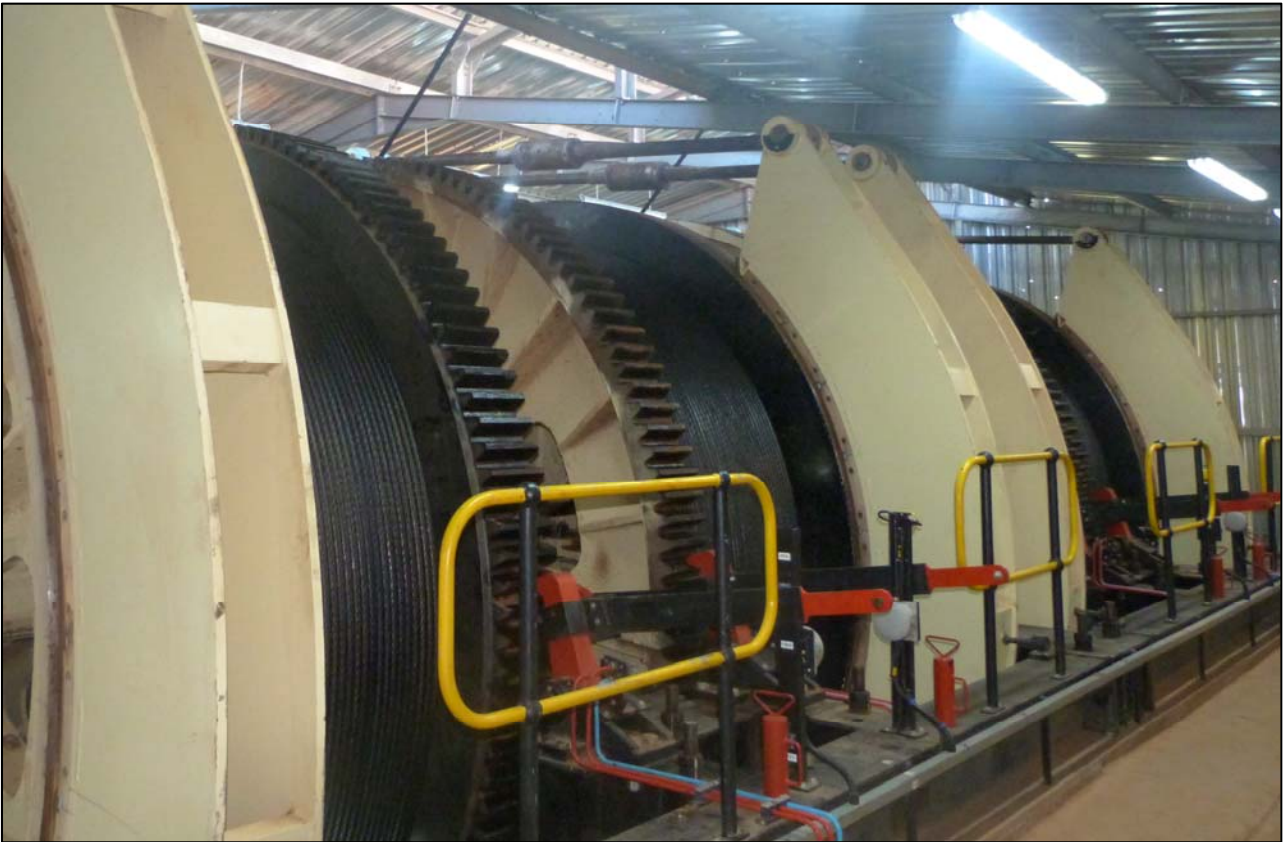
Figure 5: Rope-up complete from stage winder drums to headgear and five-deck stage on Shaft 1.
