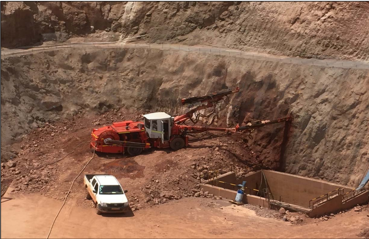
Figure 15: Installed mesh and three-metre rebar bolts.
