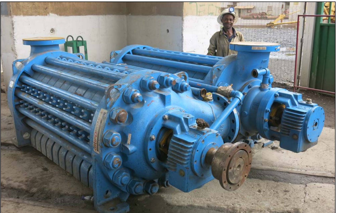
Figure 13: New Grifo centrifugal pumps to be installed at the 1,200-metre-level pump station in Shaft 5.
