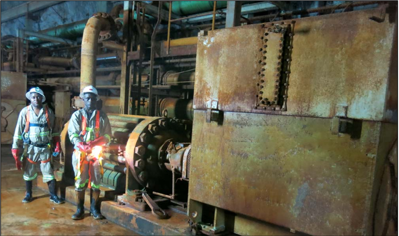
Figure 13: New Grifo centrifugal pumps to be installed at the 1,200-metre-level pump station in Shaft 5.
