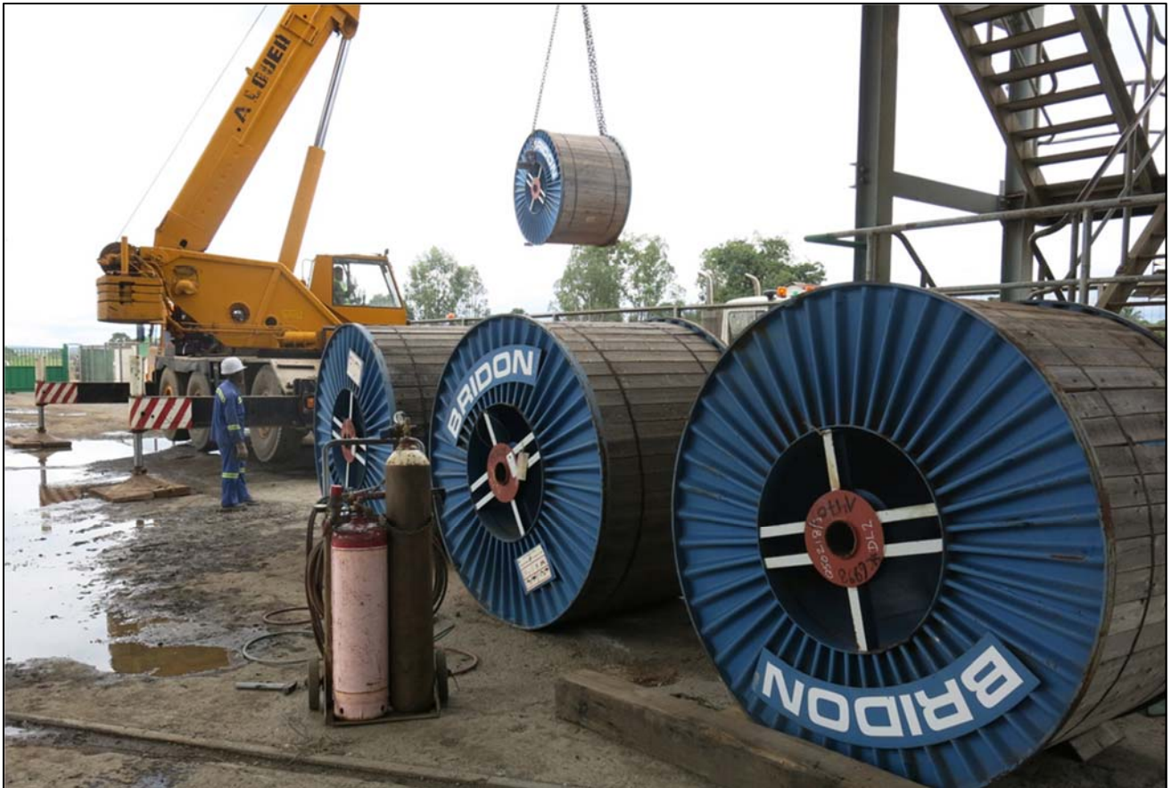
Figure 14: Delivering the new cable for the Shaft 5 man winder.
