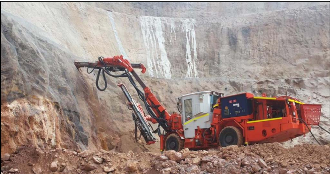
Figure 18: Drilling of anchor-bolt holes at the Kamoja box cut.
