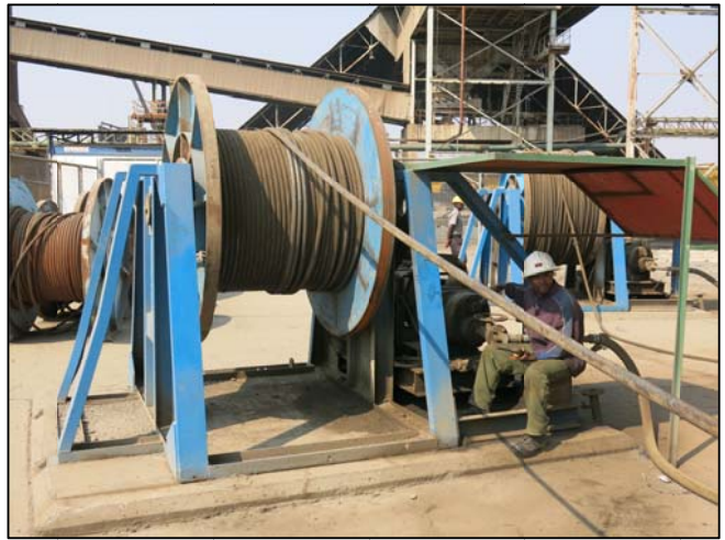
Figure 10 (right): Shaft P5 rope take-up spool during testing of refurbished gearbox.
