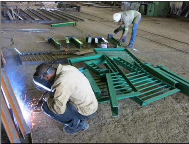
Figure 9 (left): Fabrication of platforms and ladders for emergency escapes in shafts P2, P2Bis and P15.
