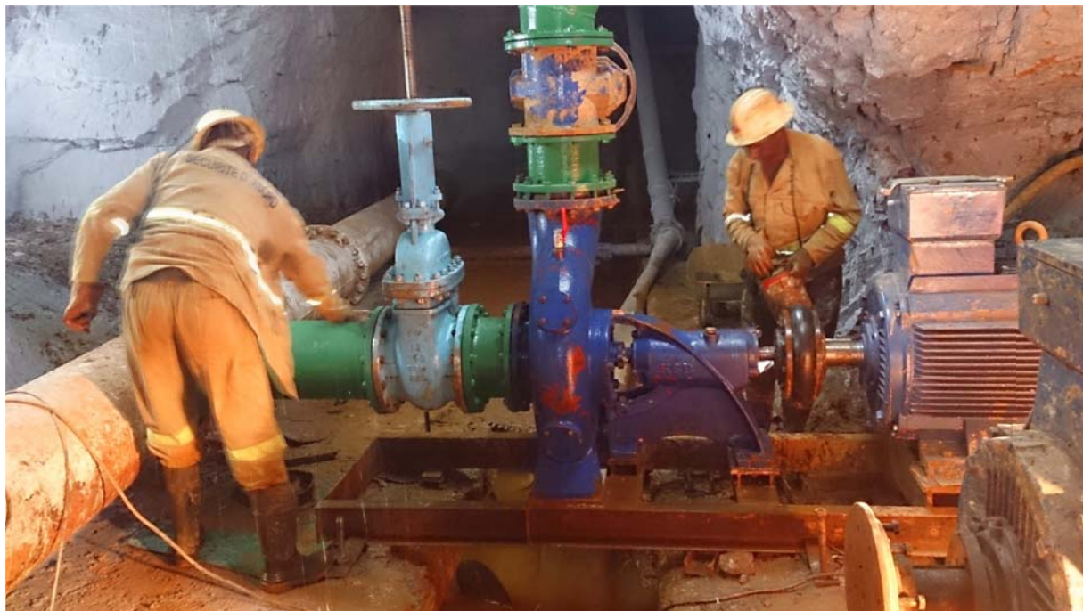
Figure 11: Testing 54-kilowatt Flygt pump in test pit.
