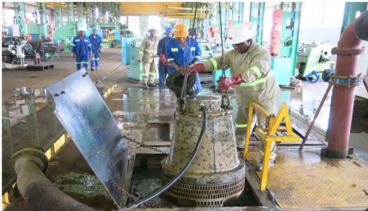
Figure 11: Testing 54-kilowatt Flygt pump in test pit.
